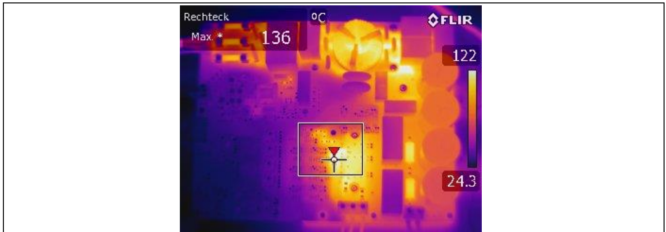
Figure 25 Thermal image of evaluation board at 18 kHz switching frequency
