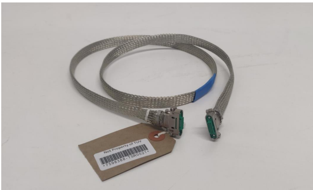
Figure 1.3.2 Equipment Under Test: Braided cable with back shells - 16-way cable assembly
