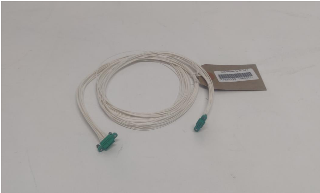
Figure 1.3.1 Equipment Under Test: Base Cable - 16-way cable assembly
