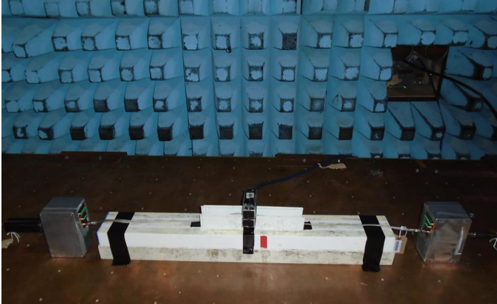
Figure 2.1.3 Test Setup: Braided cable assembly with unscreened back shells
