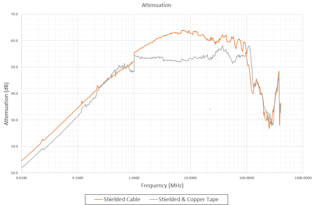
Figure 2.1.8 Attenuation achieved: Braid shielded cable with screened back shells V Shielded Cable with unscreened back shells.
