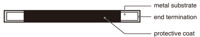
Fig. 2 The structure of a metal plate current sensor. The whole resistor body will be in contact with the PCB after mounting due to its flat design.
