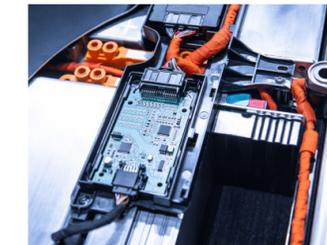
Battery management systems require bidirectional and very high precision current sensing to minimize energy losses. The sensing rate is usually low, and both high-side and low-side can be adopted. Isolated current sensing is not required up to 48V.
