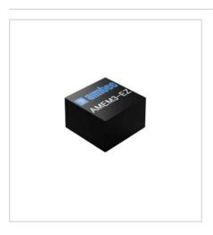
AMEM3-EZ series is an efficient 3W AC-DC power supply module. Offering a commercial input voltage range from 90VAC to 264VAC, output voltage ranges from 3.3V to 48V, and safer isolation.
