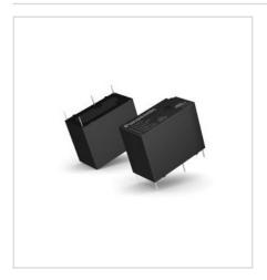
The increasing degree of automation especially for motor or LED lighting control demands switching solutions with high inrush current capability. ALQ6 type, a member of the LQ relay family, can handle an inrush current up to 40A for 100µs for a capacitive load in the same small housing as the standard version. Moreover, ALQ6 offers increased creepage and clearance distance between contact and coil of minimum 5.5mm which helps to meet various safety standards.
