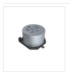
FC series Supercapacitors, also known as Electric Double-Layer Capacitors (EDLCs), are surface mount type components intended for high energy storage applications. The FC series is designed specifically for reflow soldering, allowing them to be attached to a printed circuit board (PCB) directly. This FCR type is a surface mount supercapacitor with an operating temperature range of 85°C in high temperature environments.
