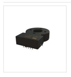
The FG-R01 series sensor is a high-sensitivity AC and DC leakage current sensor with individual open drain alarms and an analog output for leakage current indication. In addition, its integrated test coil can be initiated by a test input to perform a functional alarm test. The UL 2231 version (\*4GA) contains 2AC alarms to comply with CCID5 and CCID20.
