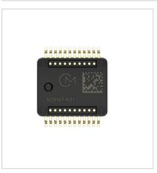
The SCH16T-K01 is a combined high-performance 3-axis angular rate and 3-axis accelerometer. The angular rate and accelerometer sensor elements are based on Murata's proven capacitive 3D-MEMS technology. Signal processing is done by a single mixed-signal ASIC that provides angular rate and acceleration via a flexible SafeSPI v2.0 compliant digital interface. Sensor elements and ASIC are packaged to pre-molded SOIC 24-pin plastic housing that guarantees reliable operation over the
