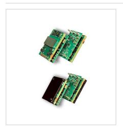
MPS0117V2NBC is a highly efficient, 200W, isolated DC-DC converter that converts 36Vdc-75Vdc input into an isolated regulated 12Vdc/17Amp output. The MPS0117V2NBC is fully protected from overcurrent, overtemperature, and overvoltage faults and is packaged within the industry standard sixteenth-brick format with baseplate. Cooling options for all applications. Safety features include 2,250Vdc I/O isolation with basic insulation suitable for POE applications.
