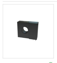
The FG-R05 series sensor is a high-sensitivity AC and DC leakage current sensor with individual open drain alarms and an analog output for leakage current indication. In addition, its integrated test coil can be initiated by a test input to perform a functional alarm test. The UL 2231 version (\*4GA) contains 2AC alarms to comply with CCID5 and CCID20.
