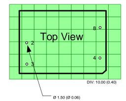
Dimensions mm (inch) Case Tolerance ±0.50 (±0.02) Pin Diameter  $1.0 \pm 0.10 (0.04 \pm 0.004)$
