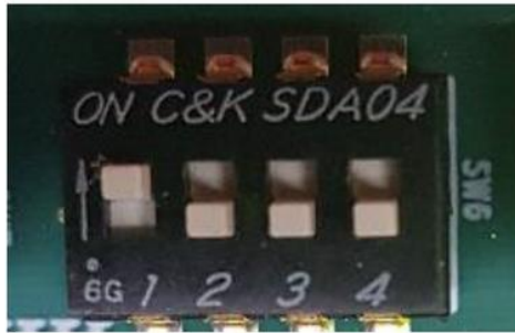
Figure 2 - ZCU111 SD boot switch settings
