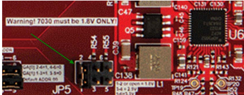
Figure 2 - Jumper Setting for 1.8V Selection
