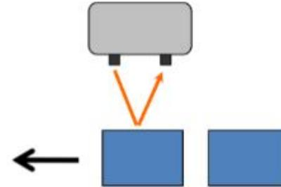
Smaller distance between sensor and object make signal bigger.
