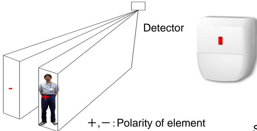
Dual element has the advantage in detection of motion across the detection area.
