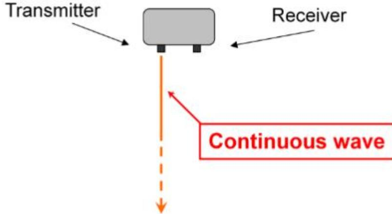
Received signal will not appear in the case that no object reflects the wave.
