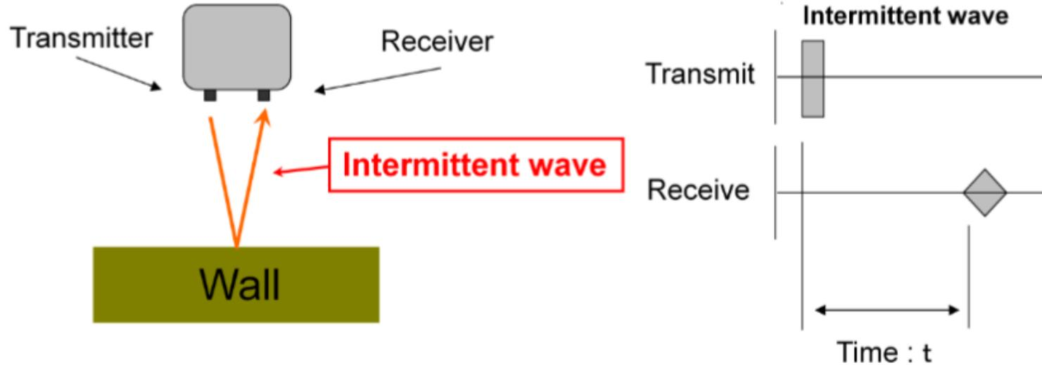
Measuring the time from transmitting to receiving (using clock)
