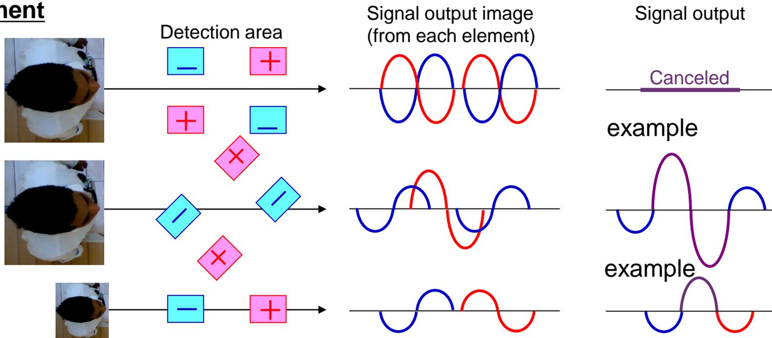
Quad element has the advantage in **the fine motion detection** when it is used in a ceiling mount detector. This performance comes from the **arrangement of element polarity and number of detection area.**
