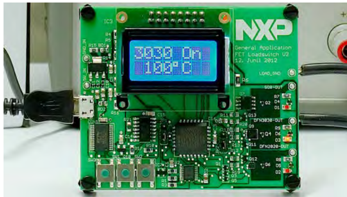
Fig 11. Test with DFN3333-8 (SOT873-1) package
