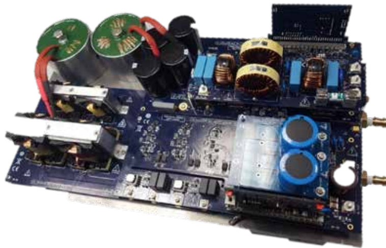
Figure 6: The 7kW On-Board Charger module demonstrates the capability of SiC and silicon MOSFET, driver, thyristor, and SPC58 microcontroller technologies
