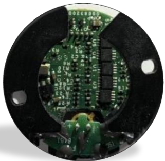
LED Driver PCB (with additional 50+ components)
