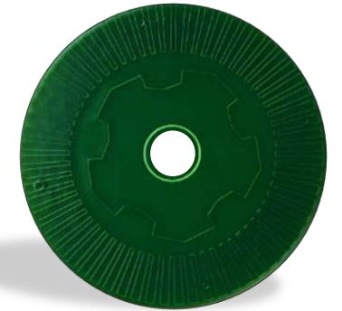
Rotor PCB (single layer, no components)
