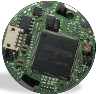
Stator PCB (with 50+ components)
