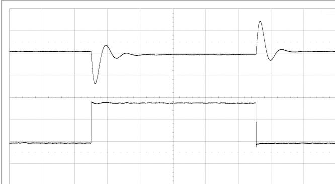
Output voltage response to load current
