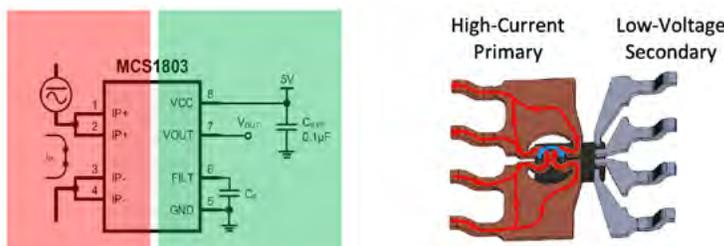
**Figure 3: High-Voltage Isolation in Standard SOIC Package**
