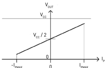
**Figure 2: Output Voltage Proportional to Primary Current**
