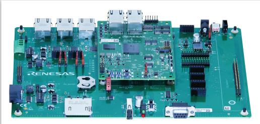
RZ/N1D-DB CPU Board mounted on the RZ/N1-EB Expansion Board
