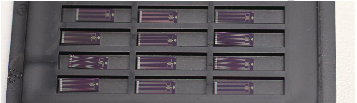
Fig. 7: SFS sensors in chip tray
