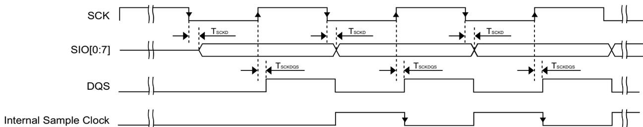
**Figure 21. FlexSPI input timing in SDR mode where FlexSPI<sub>n</sub>\_MCR0[RXCLKSRC] = 0x3 (case A2)**
