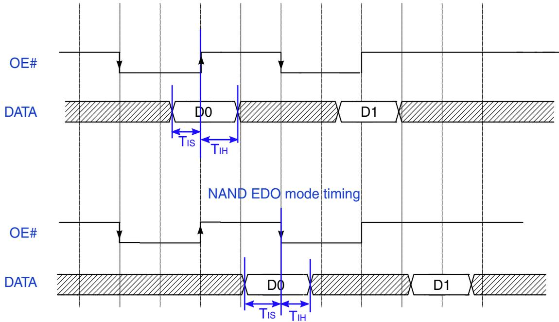
Figure 17. SEMC input timing in ASYNC mode
