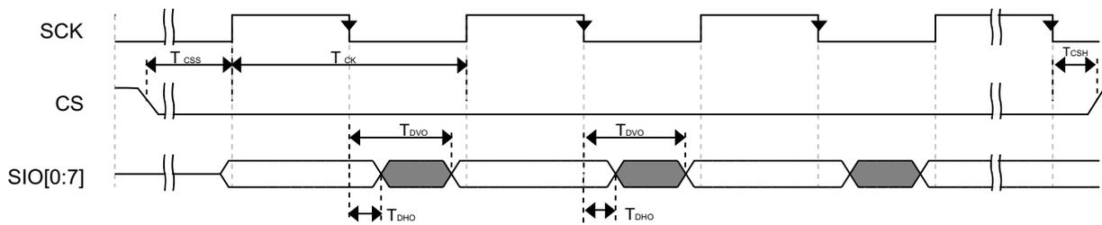
Figure 25. FlexSPI output timing in SDR mode
