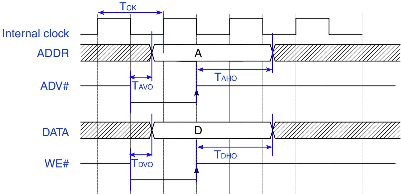
Figure 15. SEMC output timing in ASYNC mode
