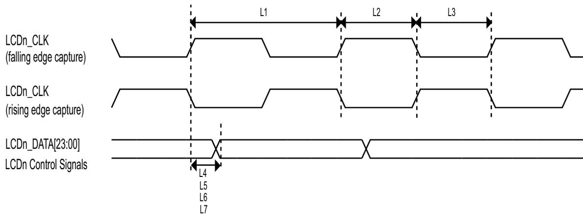
Figure 30. LCD timing
