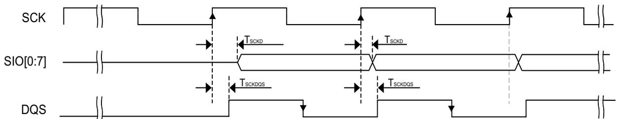
**Figure 20. FlexSPI input timing in SDR mode where FlexSPI<sub>n</sub>\_MCR0[RXCLKSRC] = 0x3 (case A1)**
