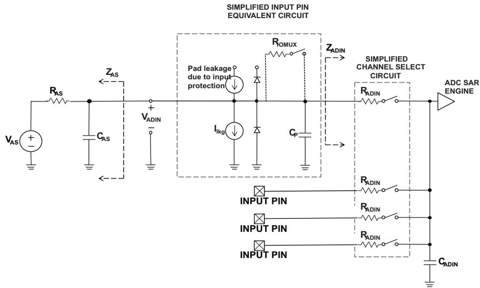
Figure 34. ADC input impedance equivalent circuit diagram
