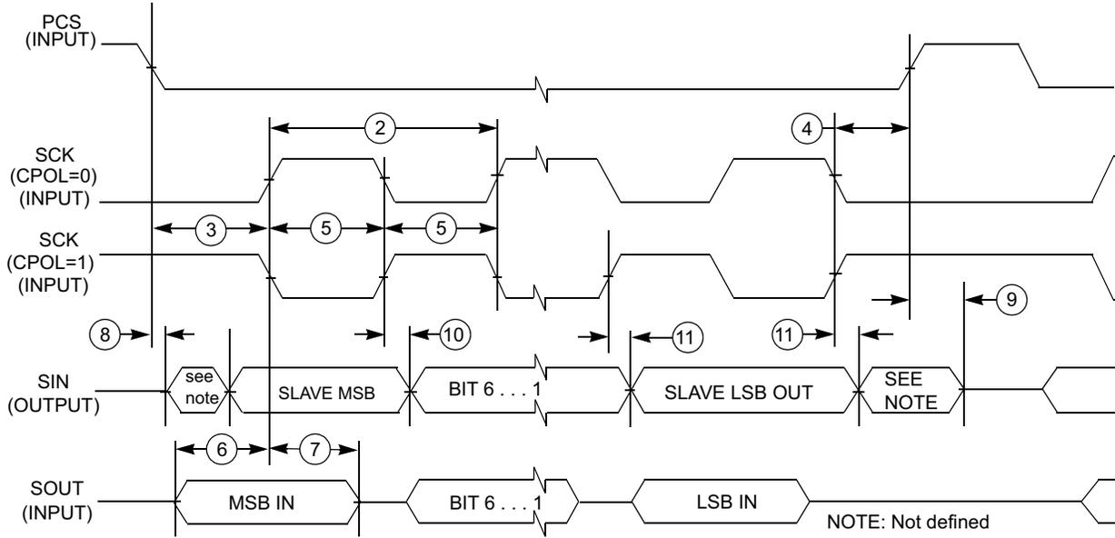
Figure 37. LPSPI Slave mode timing (CPHA = 0)
