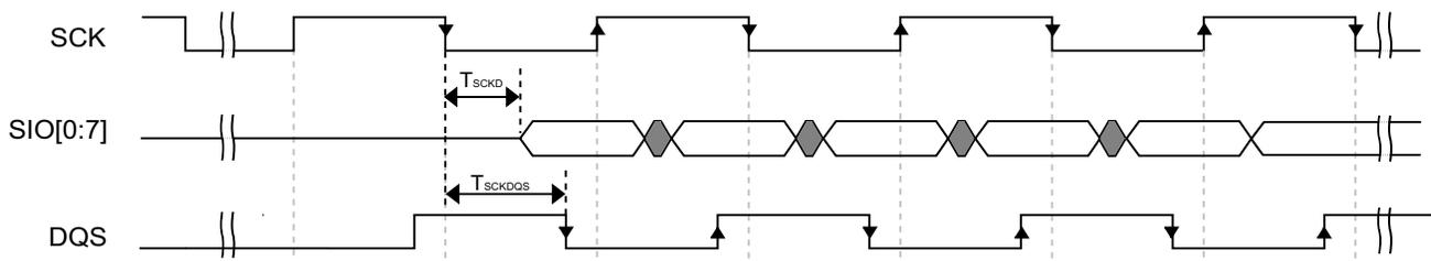
**Figure 23. FlexSPI input timing in DDR mode where FlexSPI<sub>n</sub>\_MCR0[RXCLKSRC] = 0x3 (case B1)**
