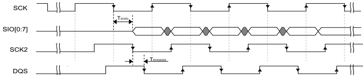
Figure 24. FlexSPI input timing in DDR mode where FlexSPI<sub>n</sub>\_MCR0[RXCLKSRC] = 0x3 (case B2)
