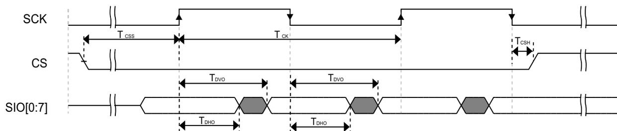
Figure 26. FlexSPI output timing in DDR mode
