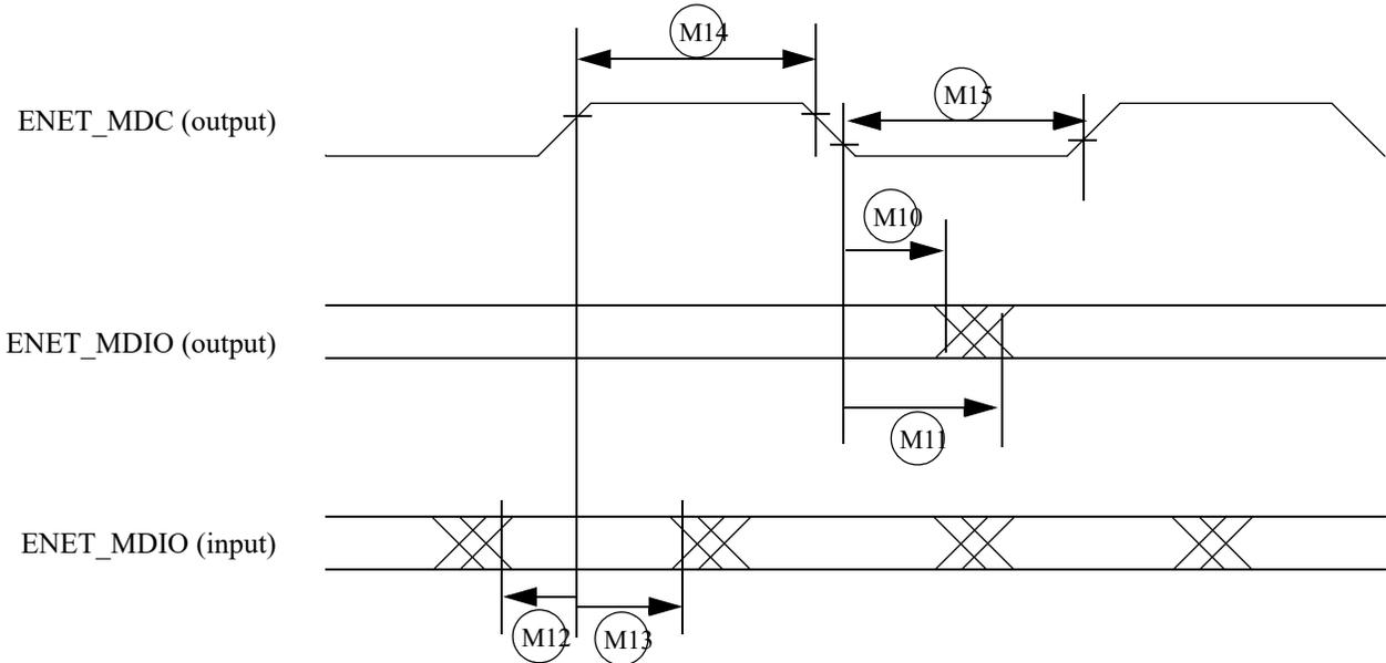
Figure 47. MII serial management channel timing diagram
