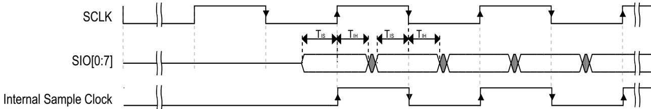
**Figure 22. FlexSPI input timing in DDR mode where FlexSPI<sub>n</sub>\_MCR0[RXCLKSRC] = 0x0, 0x1**
