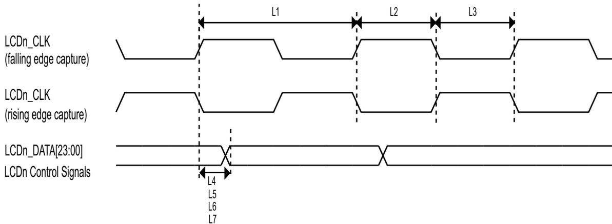
Figure 30. LCD timing
