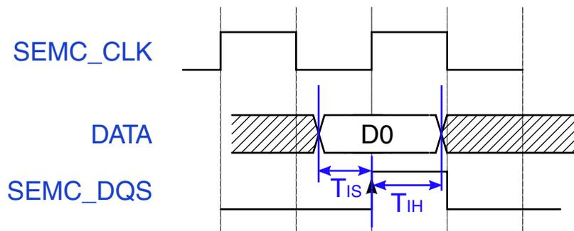
Figure 18. SEMC input timing in SYNC mode
