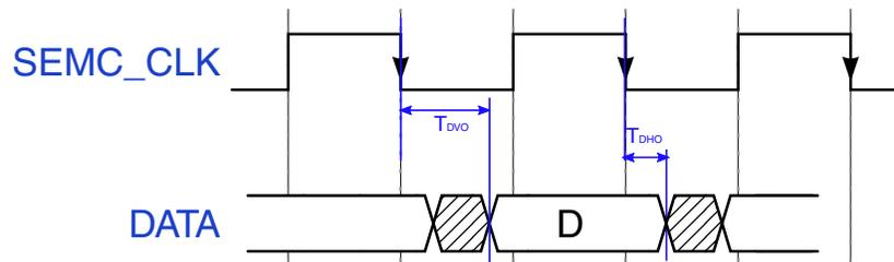
Figure 16. SEMC output timing in SYNC mode
