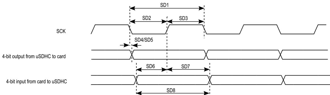
Figure 41. SDR50/SDR104 timing
