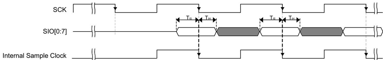
Figure 19. FlexSPI input timing in SDR mode where FlexSPI<sub>n</sub>\_MCR0[RXCLKSRC] = 0x0, 0x1
