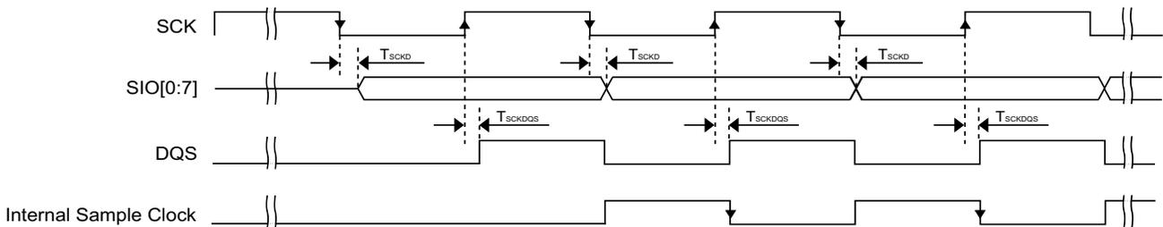
**Figure 21. FlexSPI input timing in SDR mode where FlexSPI<sub>n</sub>\_MCR0[RXCLKSRC] = 0X3 (case A2)**
