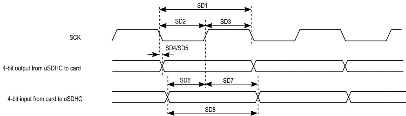
Figure 41. SDR50/SDR104 timing
