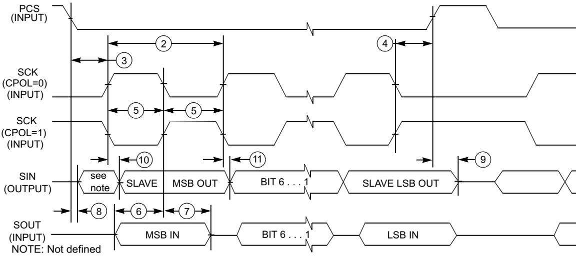
Figure 38. LPSPI Slave mode timing (CPHA = 1)
