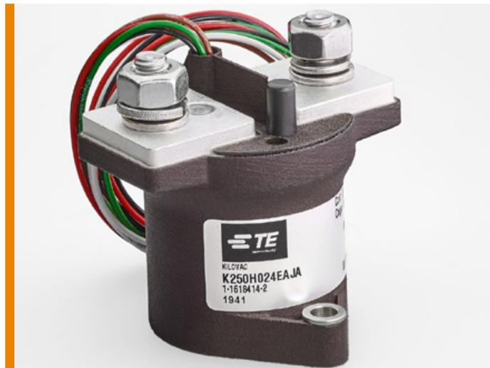
TE Connectivity (TE)'s K250 high voltage DC contactor is hermetically sealed and designed for harsh environments. It is rated at 250A continuous, with an isolation voltage of 1000VDC, offering bi-directional power switching capability. Additional key features include an electronic coil economiser for low power holding capability, as well as auxiliary contacts in a smaller size, lighter weight package.
