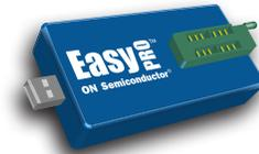
tool for ON Semiconductor serial EEPROMs (I<sup>2</sup>C, SPI, Microwire)
