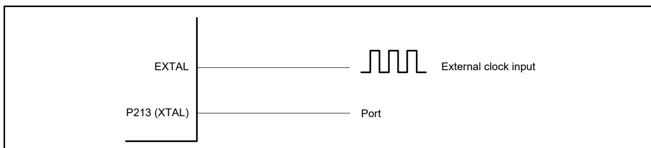
Figure 9.8 Equivalent circuit for external clock
