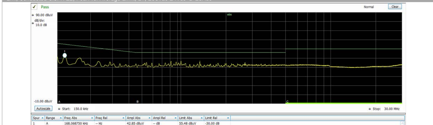
EMI; Conducted CISPR 22; Peak vs. Average Limit; L2/Neutral; 208Vac 24Vdc @ 25Acd
