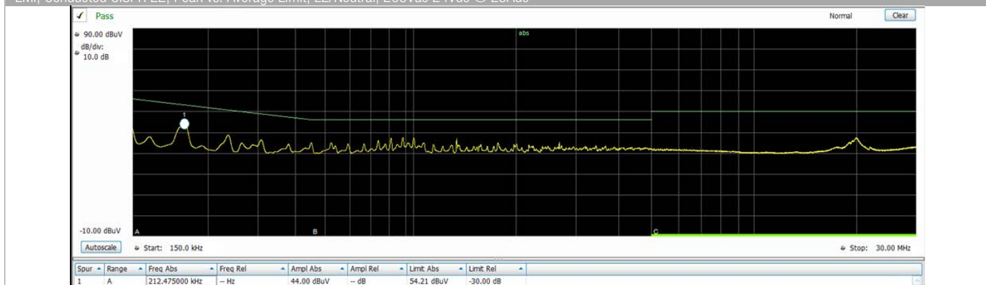
EMI; Conducted CISPR 22; Peak vs. Average Limit; L2/Neutral; 208Vac 24Vdc @ 25Acd
