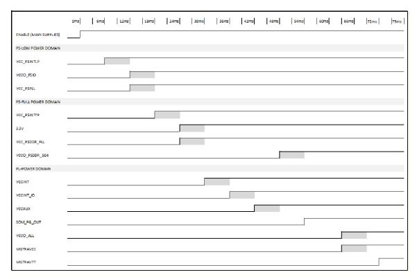
Figure 15 - UltraZed Power-On Sequence
