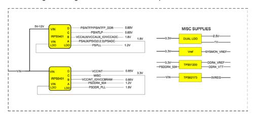
Figure 14 - On-Board Regulation Circuits
