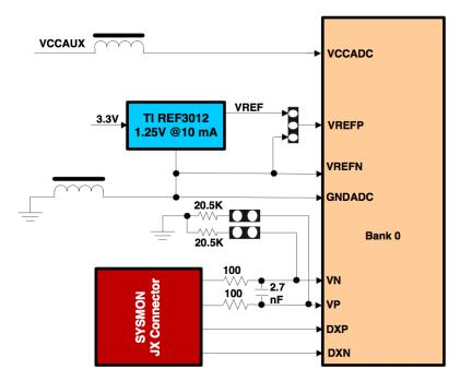
Figure 19 - UltraZed-EG SOM SYSMON Circuit
