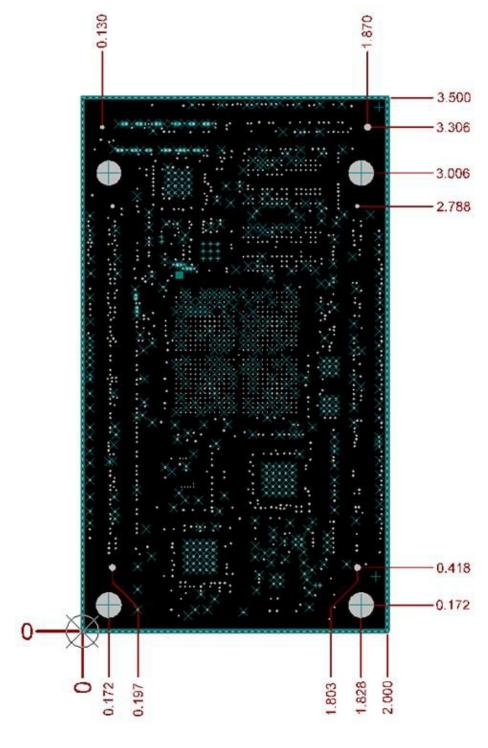
Figure 21 – UltraZed-EG SOM Top View Mechanical Dimensions
