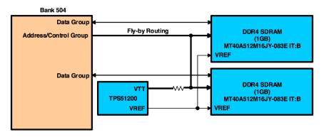
Figure 3 - DDR4 Block Diagram
