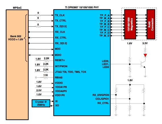
Figure 6 – 10/100/1000 Ethernet Interface Implementation
