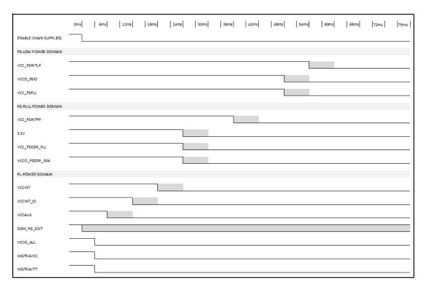
Figure 16 - UltraZed Power-Off Sequence
