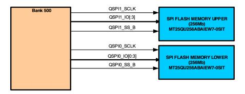
Figure 4 – Dual QSPI Block Diagram
