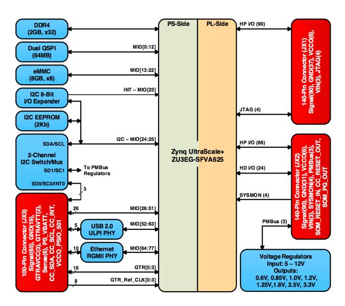
Figure 2 – UltraZed-EG SOM Block Diagram
