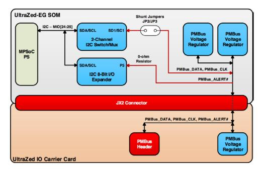
Figure 10 – PMBUS Connections
