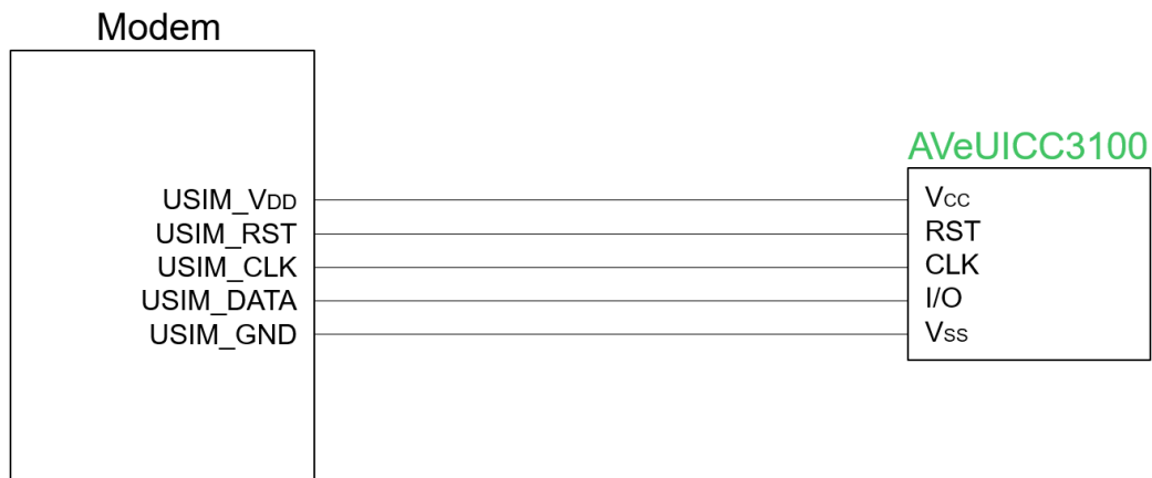
Figure 6: Typical connection to modem
