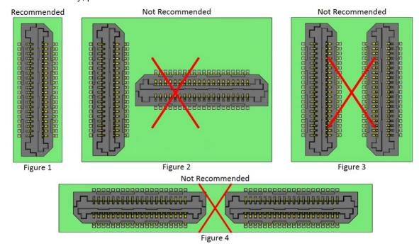
If multiple LSXX connectors per board are required, the below recommendations must be followed:
