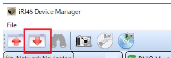
Figure 3.8 Write Configuration
