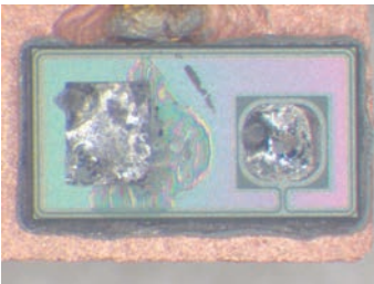
Fig 59. Sample image 68; 20 V, 3 A, 60 ms
