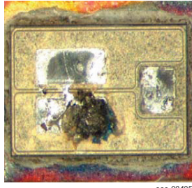
Fig 72. Sample image 14; 15 V, 5 A, 1 ms
