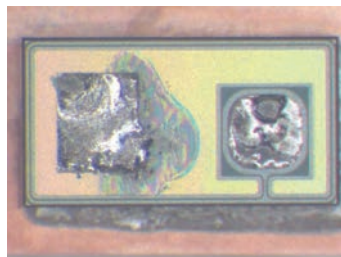
Fig 62. Sample image 72; 30 V, 1.4 A, 60 ms
