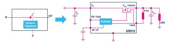
When an overload or short-circuit condition occurs, the eFuse limits the current to a pre-defined safe value. When an overvoltage condition occurs, the eFuse clamps the output voltage to a safe level, thus protecting the load from abnormalities caused by malfunctioning power supplies.
