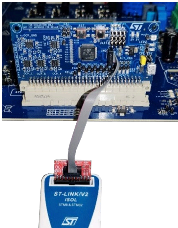
Figure 21. ST-LINK/V2 connected to the control board
