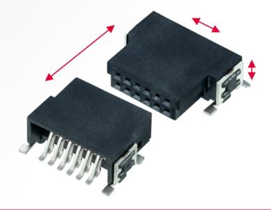
The female connector has a contact height at 1.45mm behind the mating face; the male pin is 4mm long. This gives a good tolerance to working at partially unmated conditions – the connectors will function with up to 1.5mm separation. In addition, the long twin beam design of the female connector and the chamfering of all front edges leads to tolerance to misalignment in all directions, including angled mating. The female contact design also assists in tolerance to vibration.
