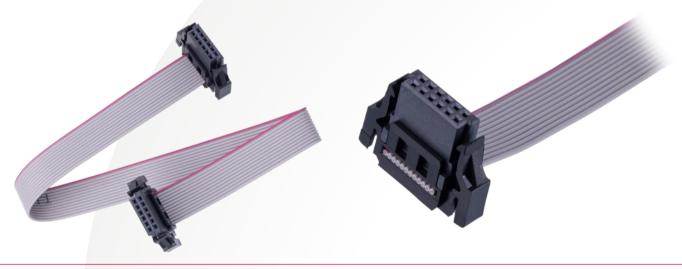
For cable to board connection, female-to-female cable assemblies are also available in the same selected sizes from 12 to 80 contacts (6+6 to 40+40). The cable length is available ready-made from stock at 150mm (6") and 300mm (12"), but other lengths can be custom-made on request (MOQs apply). UL-spec 30 AWG ribbon cable is attached via IDC to exit at right angles to the housing, and each female connector has integrated latching for additional strain relief. See M55-800 series connectors online.
