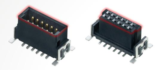
All connectors in this range feature fully shrouded and recessed contacts, to prevent accidental damage to the miniature contacts. The shrouding is also shaped to provide a positive polarization to enable assembly in only one direction.
