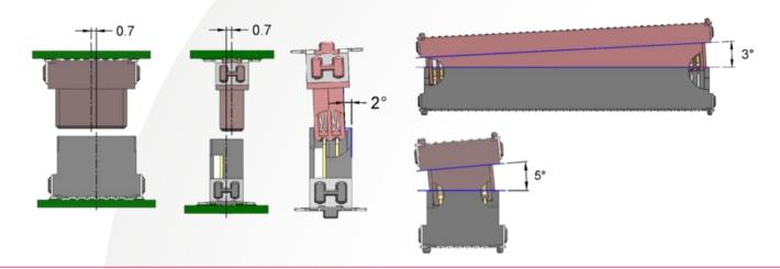
The above images show up to 0.7mm initial X and Y mating misalignment, with 2 degrees to 5 degrees angular misalignment (depending on the axis and number of contacts in the connector).
