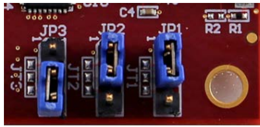
Figure 12 – MicroZed QSPI Boot Mode
