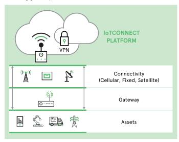
IoTConnect gateways support many interfaces, including Bluetooth, 802.15.4/ZigBee or 6LoWPAN, ModBus, CAN bus, BACnet and so on. In turn, businesses can reap the benefits of IoT by sharing data from edge devices to the cloud to reveal actionable insights that can transform business. This managed and end-to-end connectivity is made possible with:
