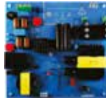
STEVAL-NRG011TV 200 W power supply based on STNRG011 digital combo for LED TV
