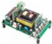
EVLMG1-250WLLC 250 W Resonant DC-DC Converter based on LCC analog controller and GaN
