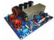
STEVAL-DPSTPFC1 3.6 kW PFC totem pole with digital inrush current limiter
