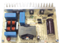
EVL6563S-250W 250 W transition-mode PFC pre-regulator
