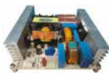
EVL4984-350W 350 W CCM PFC pre-regulator demonstration board
