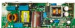
EVLCMB1-90WADP 19 V - 90 W adapter based on TM PFC and HB LLC analog combo controller
