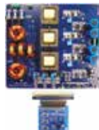
STDES-VIENNARECT 15 kW, three-phase Vienna rectifier with low cost mixed-signal control for power factor correction
