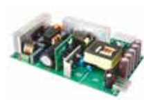
EVL400W-EUPL7 12 V - 400 W adapter based on CCM PFC and HB LLC analog controller
