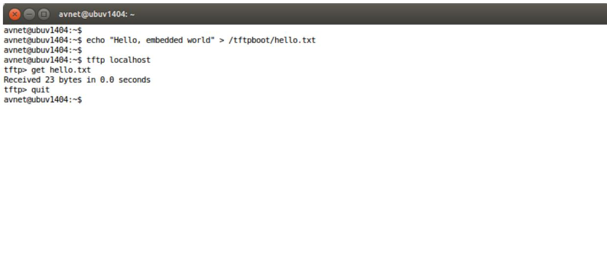
A terminal window screenshot showing the execution of TFTP commands. The terminal title is 'avnet@ubuv1404: ~'. The commands and their outputs are: 'echo "Hello, embedded world" > /tftpboot/hello.txt', 'tftp localhost', 'tftp> get hello.txt' (output: 'Received 23 bytes in 0.0 seconds'), and 'tftp> quit'.
