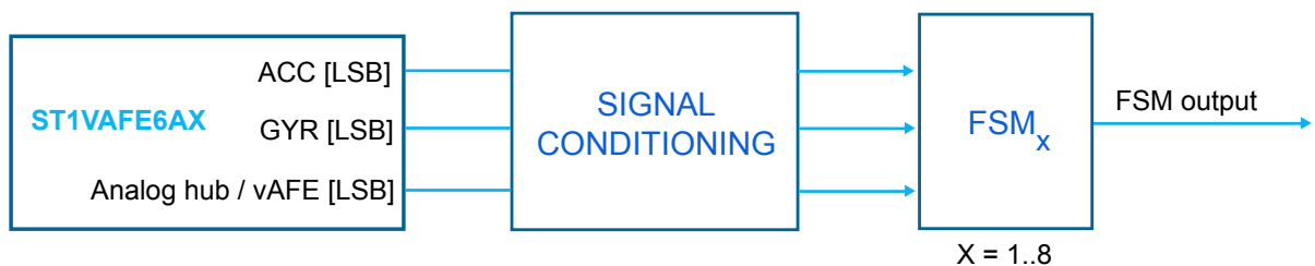
Figure 22. State machine in the ST1VAFE6AX
