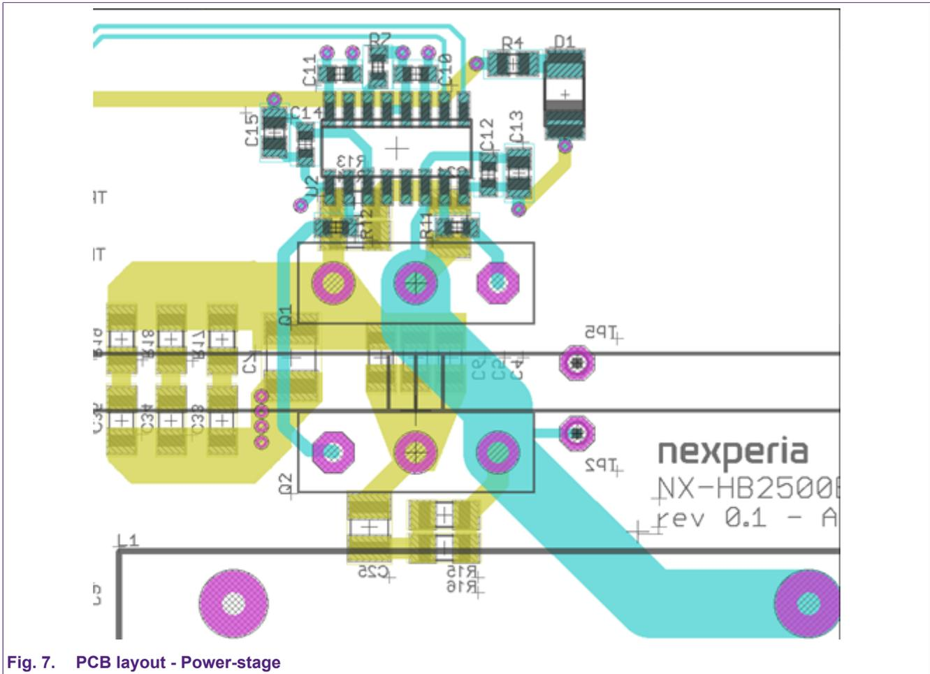
Fig. 7. PCB layout - Power-stage
