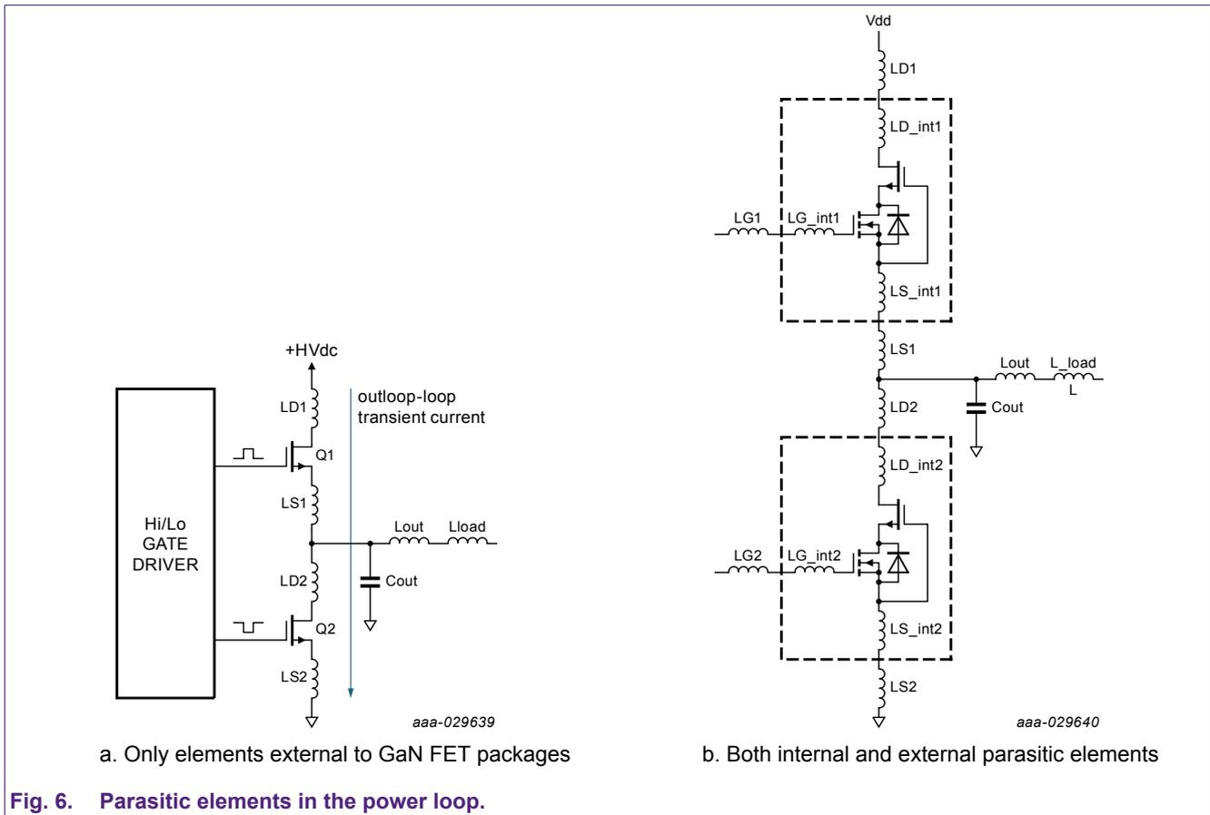
Fig. 6. Parasitic elements in the power loop.
