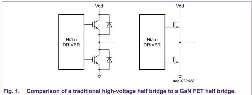
Fig. 1. Comparison of a traditional high-voltage half bridge to a GaN FET half bridge.
