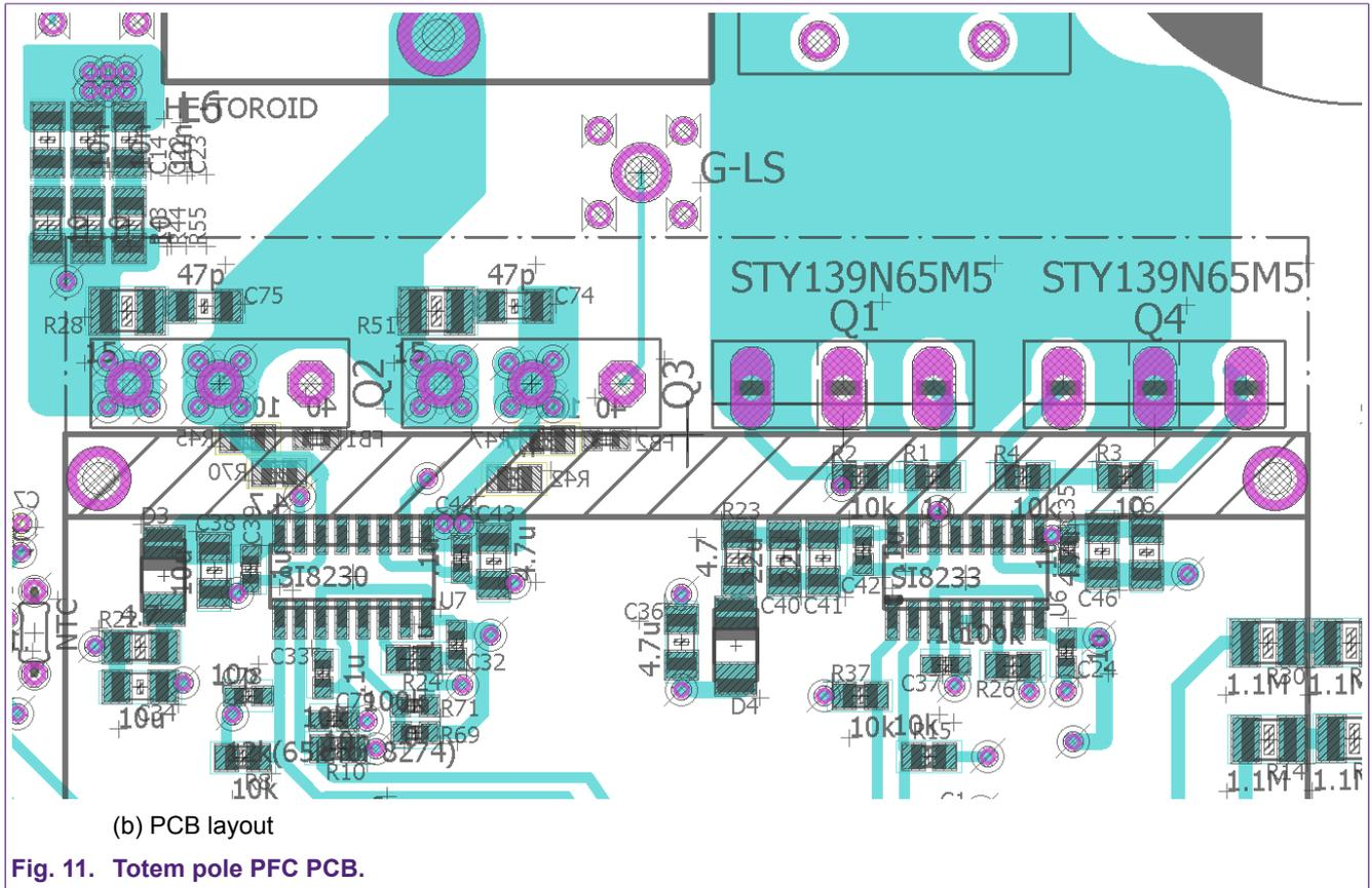
Capacitance on the switching node, indicated as  $C_{out}$  in Fig. 6, adds directly to switching loss, and so the total area of copper which forms the switching node should be kept low, but not so low that inductance becomes significant. A typical 4-layer board with 12 mils (0.3 mm) between outer trace and internal ground plane adds about 15 pF / cm<sup>2</sup>. At 100 kHz switching, each 1 cm<sup>2</sup> would add  $P = 1/2 CV^2 f_s = 120$  mW switching loss, for example.
