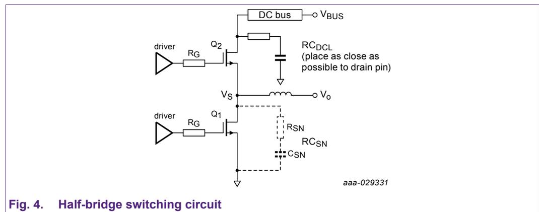
Fig. 4. Half-bridge switching circuit
