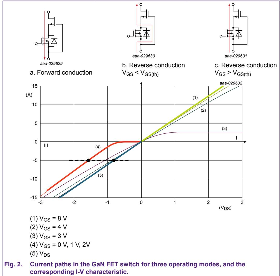
Fig. 2. Current paths in the GaN FET switch for three operating modes, and the corresponding I-V characteristic.
