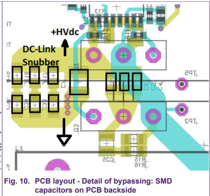
Circuit design and PCB layout recommendations for GaN FET half bridges
