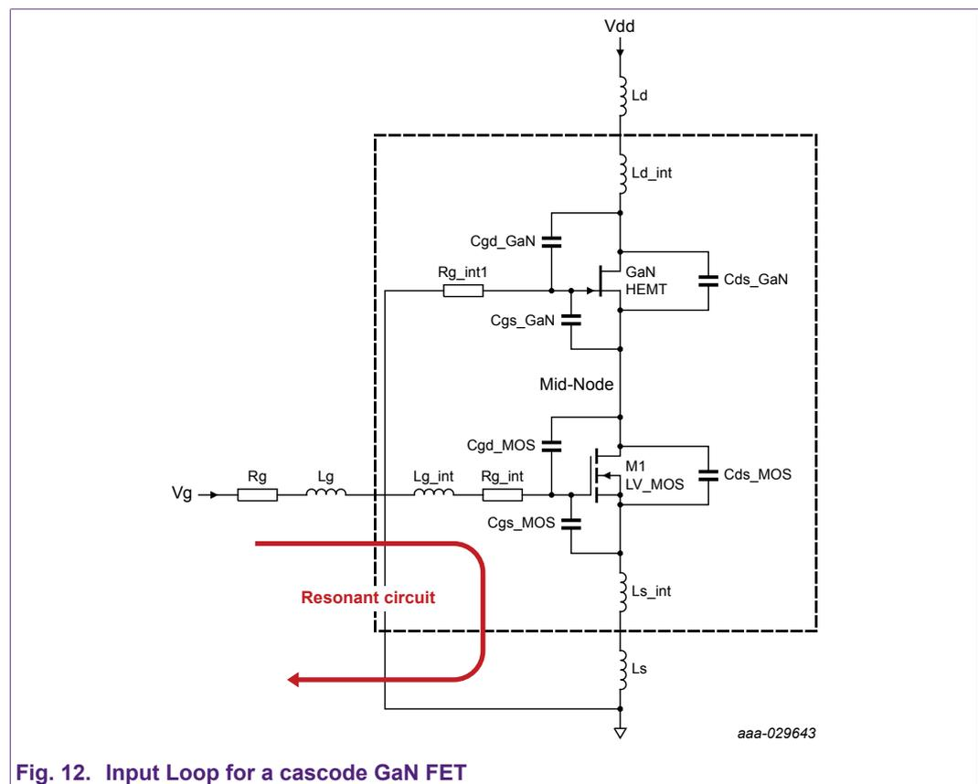
Fig. 12. Input Loop for a cascode GaN FET
