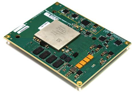
Avnet XRF™ RFSOC System-on-Modules are designed for large-scale integration into deployed RF systems demanding small footprint, low power, and real-time processing. XRF modules feature the Xilinx Zynq® UltraScale+™ RFSOC Gen-2 / Gen-3 with up to 16 RF-ADC and 16 RF-DAC channels supporting up to 6 GHz analog bandwidth.
