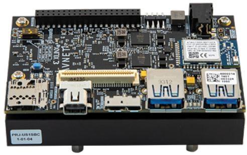
The Ultra96-V2 is an Arm-based, Xilinx Zynq UltraScale+™ MPSoC single board computer based on the Linaro 96Boards Consumer Edition (CE) specification. Ultra96-V2 is available in many countries around the world as it has been designed with a certified radio module from Microchip. Additionally, Ultra96-V2 is available in both commercial and industrial temperature grade options. Additional power control and monitoring is possible with the included Infineon PMICs.
