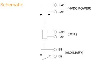
Note: Contactors should be installed so that current flows from A1 (+) to A2 (-)
