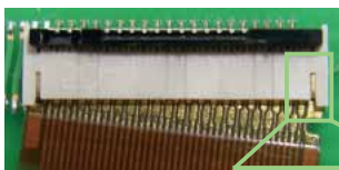
Incomplete FPC insertion
