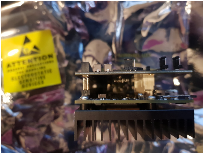
Figure 3. Aligning the high-speed and low-speed connectors
