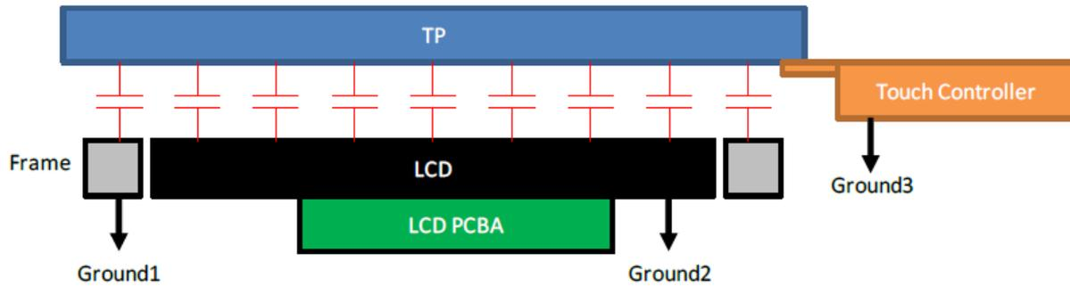
GND1, GND2 and GND3 should be connected together to have the same ground
