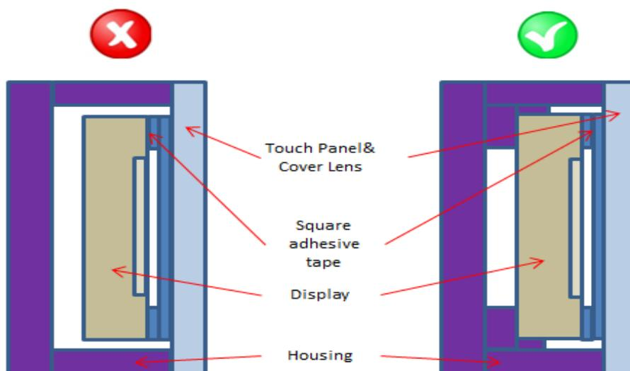
3) TP needs to work in environment with stable stray capacitance. In order to minimize the variation in stray capacitance, all conductive mechanical parts must not be floating. Intermittent floating any conductive part around the touch sensor may cause significant stray capacitance change and abnormal touch function. It is recommended to keep all conductive parts having same electrical potential as the GND of the touch controller module.
