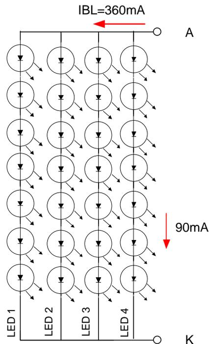
When LCM is operated over 40°C ambient temperature, the IBL should be follow :
