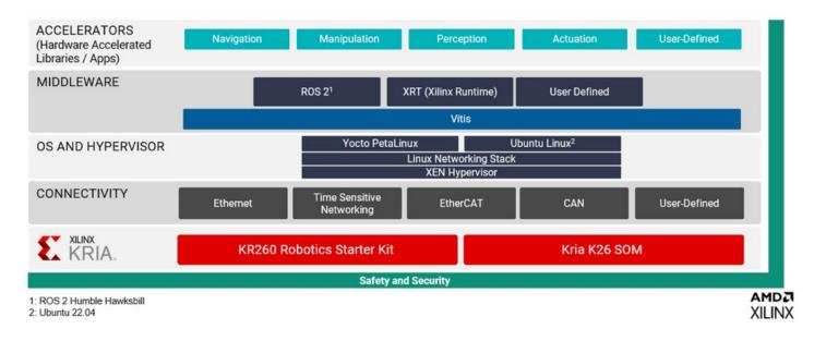
The Kria Robotics Starter Kit and KRS enable developers to create higher performance robotics solutions using familiar frameworks that address the challenges faced by modern robotic systems development.
