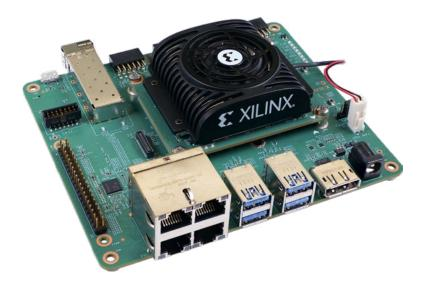
To aid development of robotic solutions, AMD Xilinx also offers the Kria<sup>™</sup> KR260 Robotics Starter Kit, which provides not only the Kria K26 SOM, but also a carrier card that contains many standard interfaces used in the development of robotic systems. The Kria Robotics Starter Kit therefore enables development of robotic applications while custom carrier cards are being developed, reducing development timescales and technical risk.
