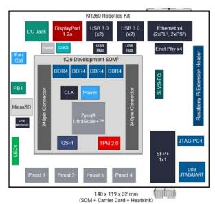
This Quad Ethernet capability with connections to both the programmable logic and the processing system enables the developer to implement time-sensitive networking if deterministic communications are required.
