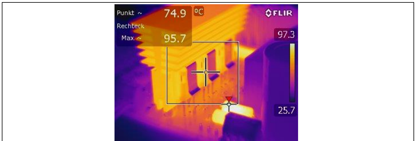
Figure 31 Thermal image of right power MOSFETs (hotspot at the capacitor's balancing resistors)
