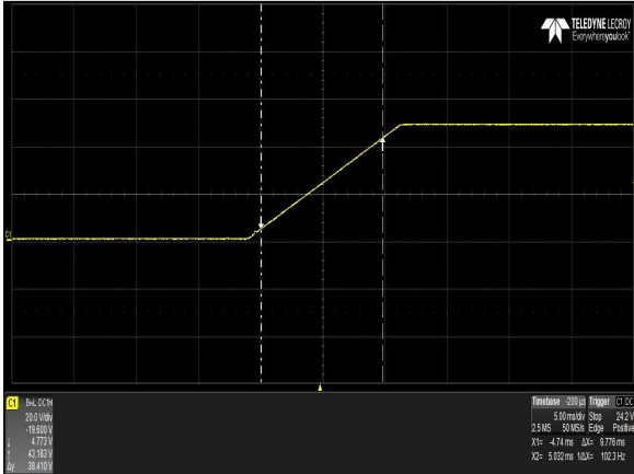
Figure 40: iHP24H3A-SW-00 Output Voltage Startup Characteristic V_{IN} = 380V_{ac} Load: I_o = 62.5A Ch 1: V_o
