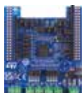
X-NUCLEO-OUT01A2 Industrial digital output expansion board based on ISO8200BQ for STM32 Nucleo
