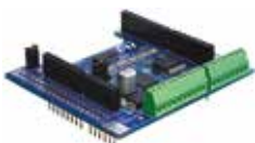
X-NUCLEO-PLC01A1 Industrial input/output expansion board based on VNI8200XP and CLT01-38SQ7 for STM32 Nucleo
