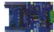
X-NUCLEO-OUT15A1 Industrial digital output expansion board based on IPS1025HF for STM32 Nucleo
