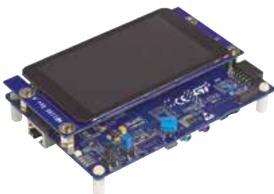
Discovery kit with high-performance STM32H7 series microcontroller with DSP and DP-FPU (STM32H7471-DISCO)
