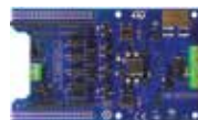
X-NUCLEO-OUT03A1 Industrial digital output expansion board based on IPS2050H for STM32 Nucleo
