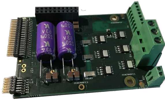
Figure 5: The Low-Voltage Power Board featuring the latest generation U-MOSIX-H TPW3R70APL MOSFETs supporting motors of up to 200 W.
