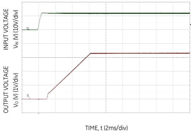
Figure 30. Typical Start-up Using Input Voltage (V<sub>IN</sub> = 12V, I<sub>o</sub> = I<sub>o,max</sub>).
