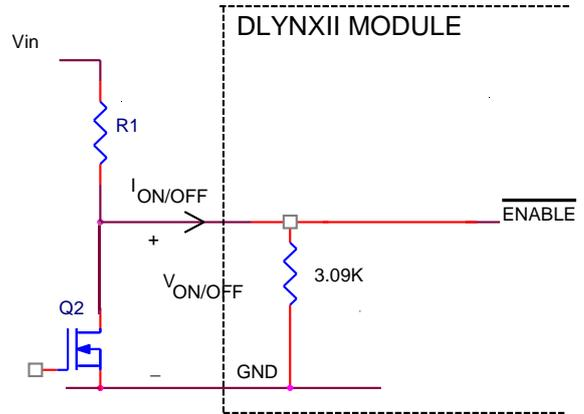
Figure 34. Circuit configuration for using negative On/Off logic.
