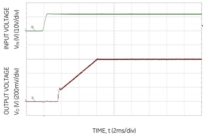
Figure 6. Typical Start-up Using Input Voltage (V<sub>IN</sub> = 12V, I<sub>o</sub> = I<sub>o,max</sub>).
