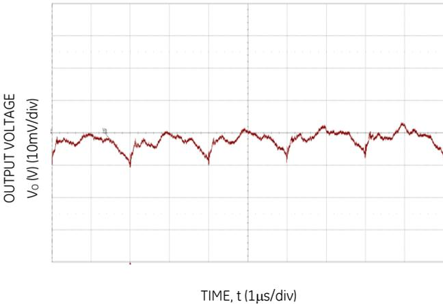
Figure 3. Typical output ripple (C<sub>o</sub>=7x22µF ceramic, V<sub>IN</sub> = 12V, I<sub>o</sub> = I<sub>o,max</sub>.)
