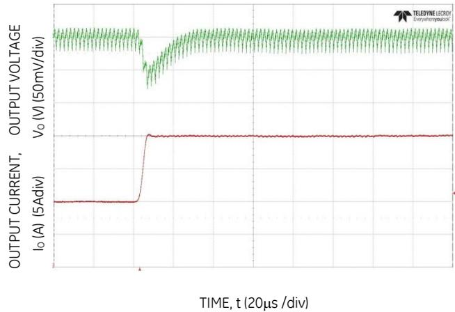
Figure 28. Transient Response to Dynamic Load Change from 50% to 100% at 12V<sub>in</sub>, C<sub>out</sub>= 4x47µF + 1x330µF, C<sub>Tune</sub>=1800pF, R<sub>Tune</sub>=300
