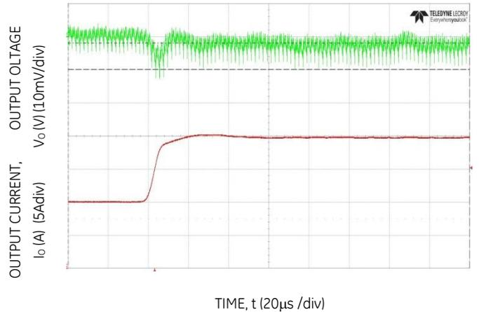
Figure 4. Transient Response to Dynamic Load Change from 50% to 100% at 12V<sub>in</sub>, C<sub>out</sub>= 7x47uF+9x330uF C<sub>Tune</sub>=15nF, R<sub>Tune</sub>=300
