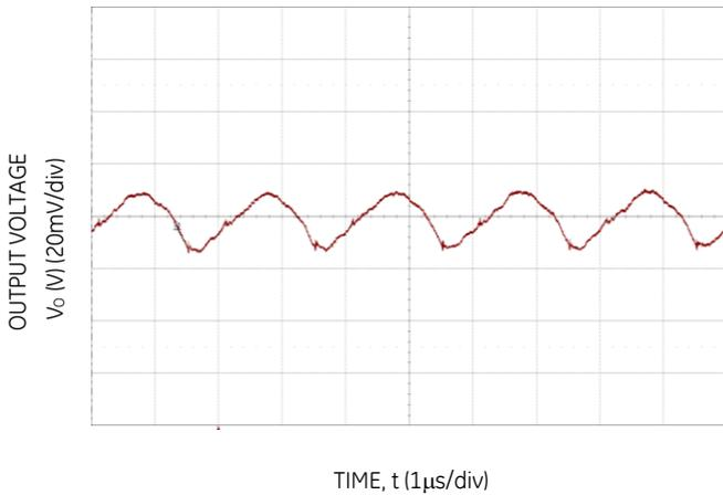
Figure 27. Typical output ripple and noise (C<sub>o</sub>=7x22µF ceramic, V<sub>IN</sub> = 12V, I<sub>o</sub> = I<sub>o,max</sub>).
