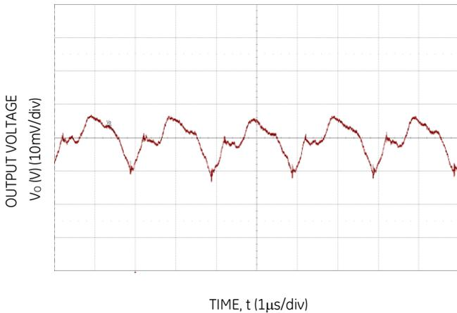
Figure 15. Typical output ripple and noise ( $C_o=7\times 22\mu\text{F}$  ceramic,  $V_{IN} = 12\text{V}$ ,  $I_o = I_{o,max}$ ).
