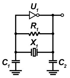
A Colpitts oscillator design, as shown below, is optimized to user a parallel resonant crystal.
