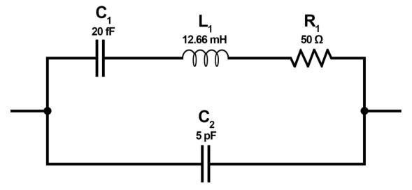
The circuit above is the electrical model of a quartz crystal, which is used in oscillators. The equivalent electrical circuit shows a series RLC circuit in parallel with a capacitance, C<sub>2</sub>. The
