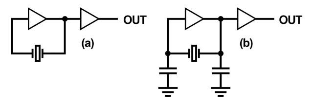
Crystal Functionality in an Electrically Equivalent Circuit
