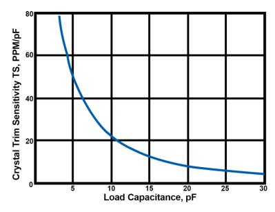
If the goal is a stable, fixed frequency oscillator, choose a crystal designed to use a large load capacitance value like 18 pF - 20 pF. To tune, or pull, the crystal, or need a low power solution, choose a crystal that uses a small load capacitance value like 8 pF - 12 pF.
