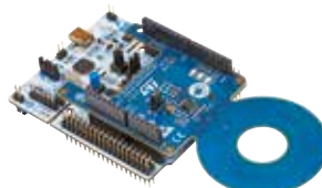
X-NUCLEO-NFC04A1 ST25DV-based NFC/RFID Dynamic Tag Nucleo expansion board
