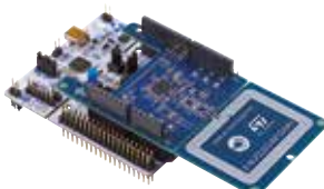
X-NUCLEO-NFC05A1 ST25R3911B-based NFC/RFID Reader Nucleo expansion board
