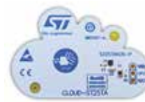
CLOUD-ST25TA ST25TA-based NFC/RFID Tag evaluation board
