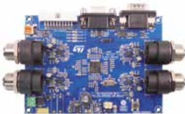
ST IO-Link demonstration kit with STEVAL-IDP004V1 on the left and STEVAL-IDP003V1D on the right.
