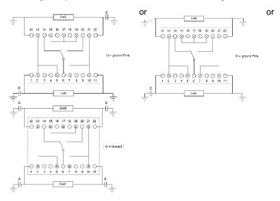
The capacitor(s) should be placed as close as possible nearby the coil-terminal(s). Good results have been obtained with RF-capable 10 pf -thin-film 603 smd-capacitors.
