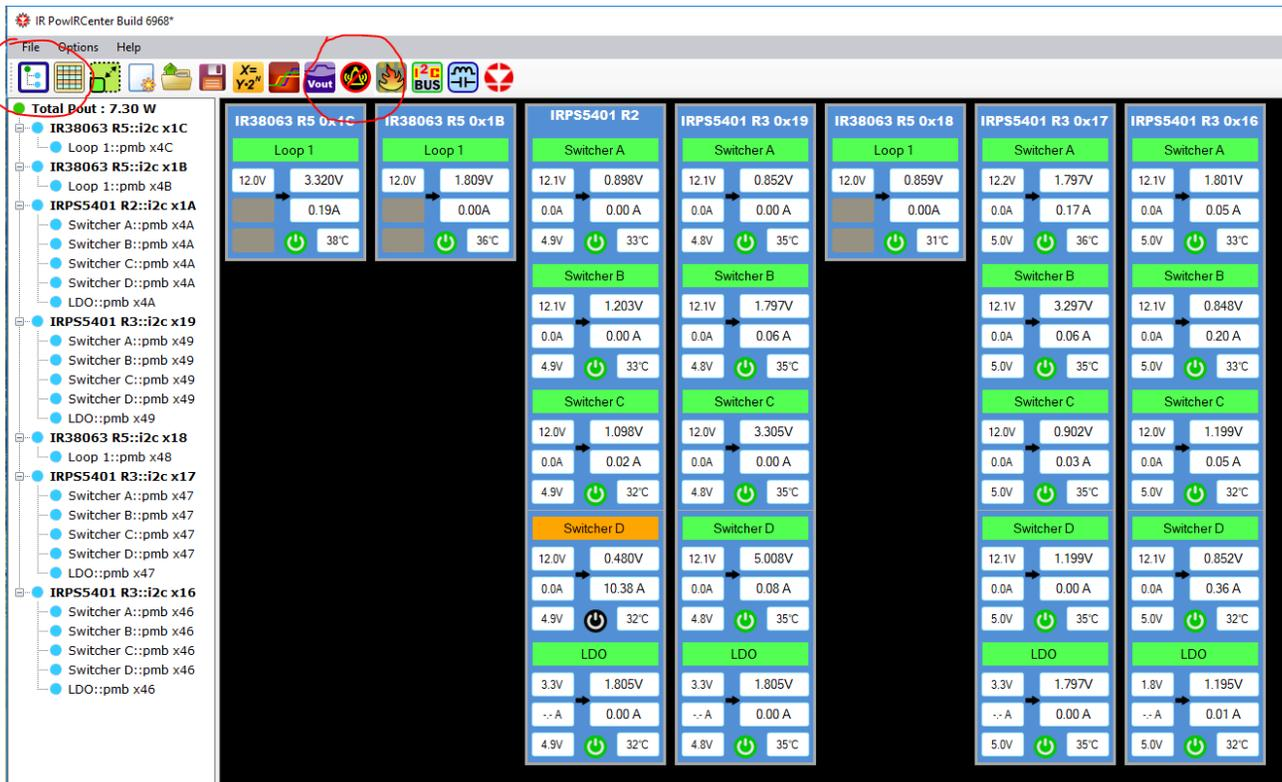
Next click on the IRPS5401 device at address x17 on the device tree on the left side. Click on the Design Wizard tab, then click on "load config file" and select the 032619\_som\_0x17.txt file to perform the update. To make sure it loads properly, click write all registers after loading the new file.
